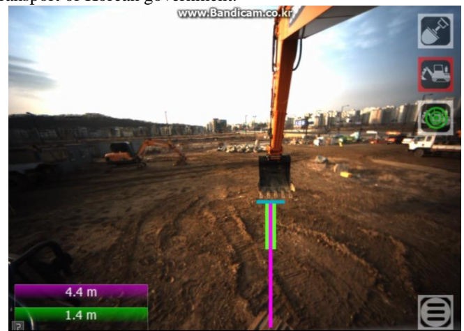
Figure 1. Edge of bucket, as-designed ground elevation, and current ground elevation shown on AR-Navigator
