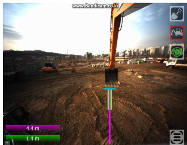
Figure 1. Edge of bucket, as-designed ground elevation, and current ground elevation shown on AR-Navigator
