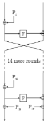
Fig 5- Feistel Structure of Blowfish Algorithm
