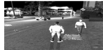
Fig. 14 –Lumigrids formed by the shirt mounted unit of a pedestrian in the guidance phase
