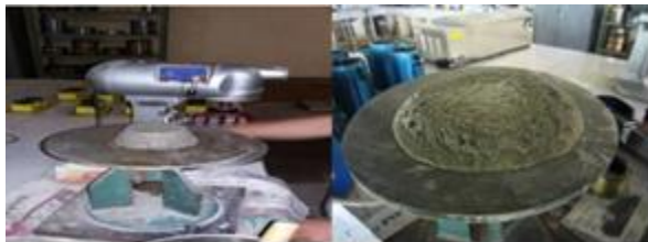
Figure 1. Flow test to measure the consistency of mortar using Flow Table.
